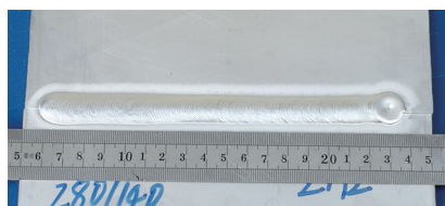
图2 Al-Cu 2#焊接接头正面外观 Fig.2 Appearance of Al-Cu 2# welded joint
